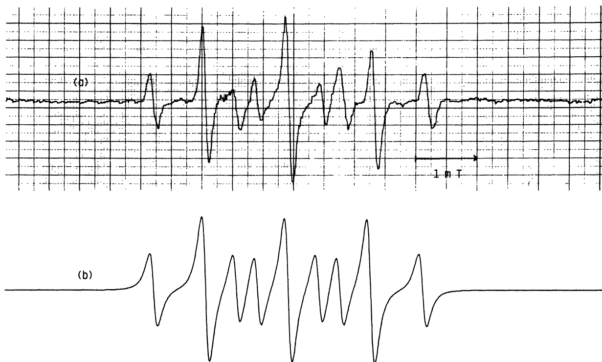
Fig. 3. ESR spectrum of spin adduct of nitrosodurene with \cdot\text{CH}_2\text{Cl} radical. Observed (a) and simulated (b) spectra.
